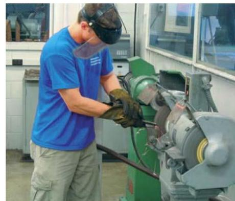
A worker using a fixed grinding wheel
