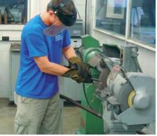
A worker using a fixed grinding wheel
